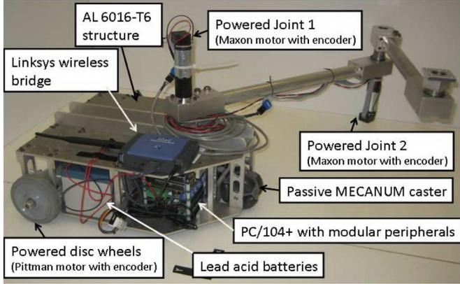
Fig. 2. Experimental electromechanical prototype of the WMM.
