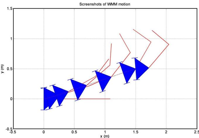
Fig. 6. Screenshots of the experimental WMM motion (from left to right, and plotting at the frame rate of 1 frame per 2.5 s).
