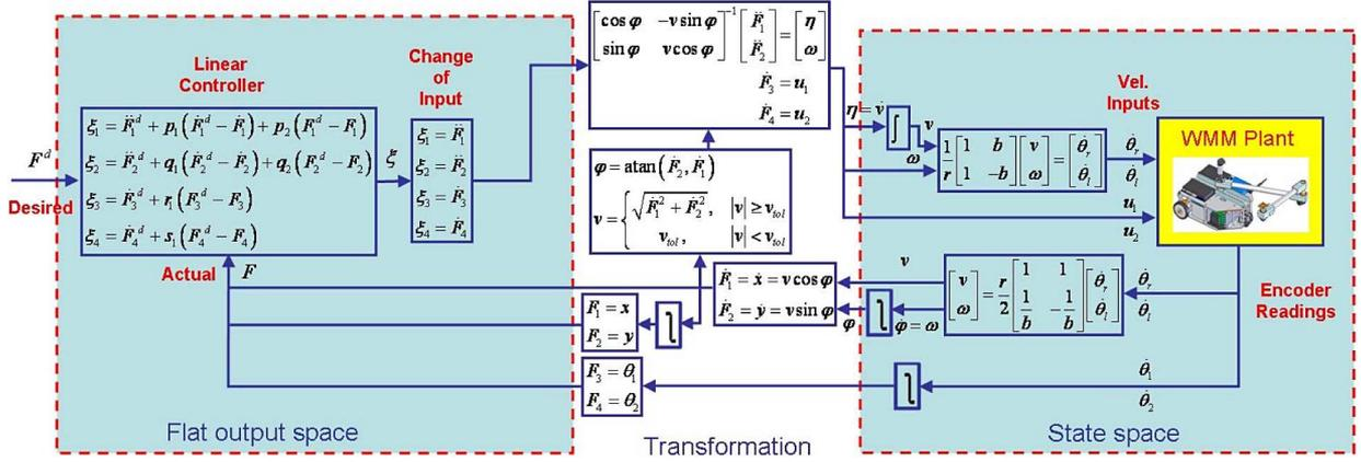
Fig. 4. Differential flatness-based control implementation framework for a WMM.
