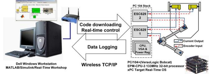
Fig. 3. MATLAB/xPC Target hardware-in-the-loop control framework.
