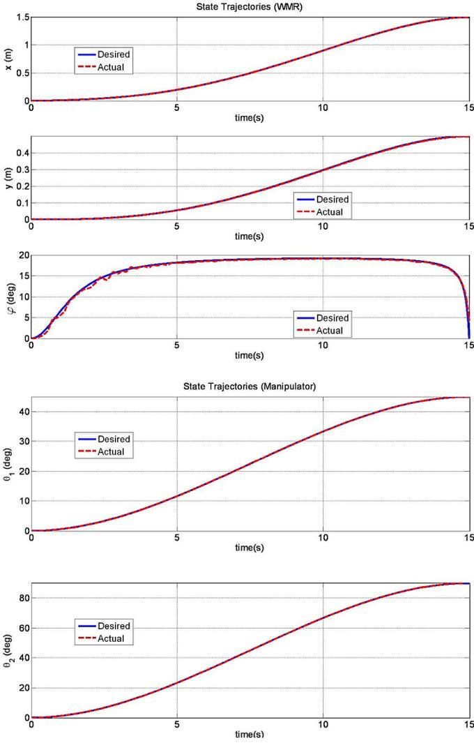
Fig. 5. Simulation and experimental results of the state trajectories  $x(t)$ ,  $y(t)$ ,  $\varphi(t)$ ,  $\theta_1(t)$ ,  $\theta_2(t)$ .
