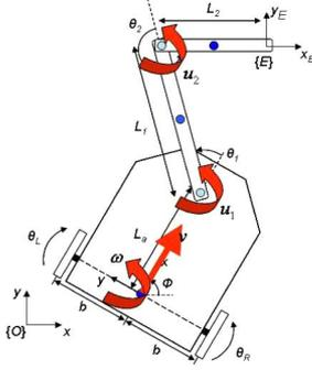
Fig. 1. Schematic of the WMM under consideration. The states are  $[x, y, \varphi, \theta_1, \theta_2]^T$ , the inputs are  $[v, \omega, u_1, u_2]^T$ , and the flat outputs are chosen to be  $[x, y, \theta_1, \theta_2]^T$ .
