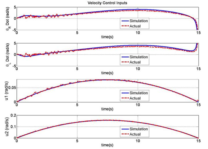
Fig. 7. Angular velocity input to each actuator  $\dot{\theta}_R(t)$ ,  $\dot{\theta}_L(t)$ ,  $u_1(t)$ ,  $u_2(t)$ .
