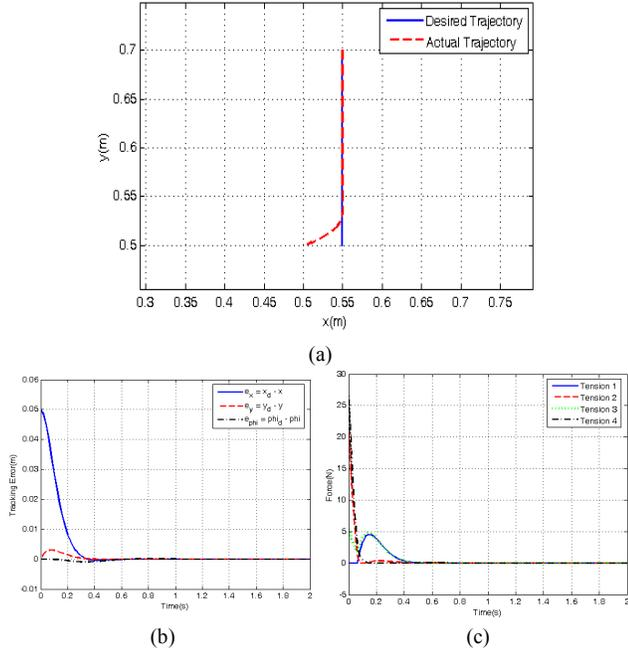
Fig. 6. Trajectory tracking performance without LBSC: (a) the desired and actual tracking trajectories; (b) the tracking errors of  $x, y, \phi$ ; and (c) the tension force in all the cables during the trajectory tracking.
