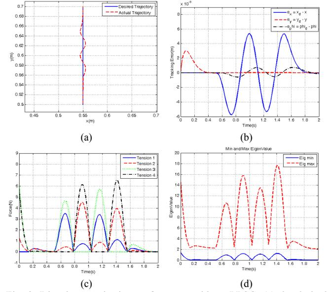
Fig. 8. Disturbance rejection performance without LBSC: (a) the desired and actual tracking trajectories; (b) the tracking errors of  $x, y, \phi$ ; (c) the tension force in all the cables during the trajectory tracking; and (d) the evolution of the maximum and minimum eigenvalues of the stiffness matrix.
