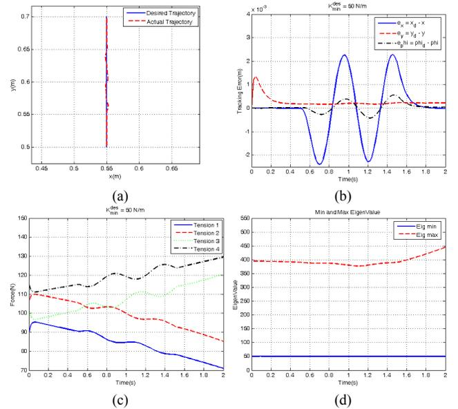
Fig. 9. Disturbance rejection performance with LBSC: (a) the desired and actual tracking trajectories; (b) the tracking errors of  $x, y, \phi$ ; (c) the tension force in all the cables during the trajectory tracking; and (d) the evolution of the maximum and minimum eigenvalues of the stiffness matrix.
