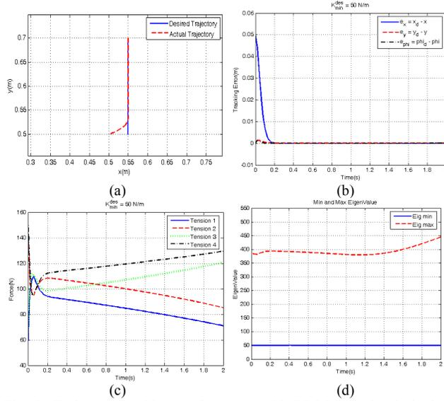
Fig. 7. Trajectory tracking performance with LBSC: (a) the desired and actual tracking trajectories; (b) the tracking errors of  $x, y, \phi$ ; (c) the tension force in all the cables during the trajectory tracking; and (d) the evolution of the maximum and minimum eigenvalues of the stiffness matrix.
